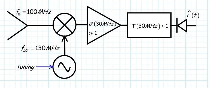
Thus, the **desired** RF signal will be **down-converted** to the IF frequency of **30 MHz**.
