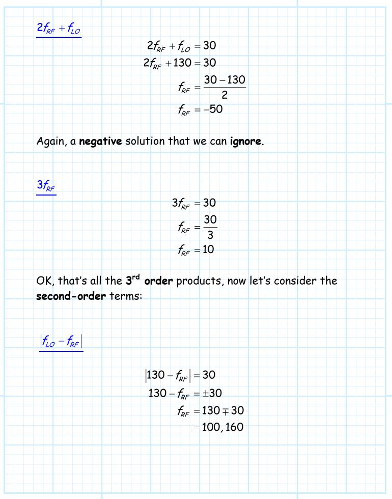
\* Note that this term is the term created by an **ideal** mixer. As a result, we find that **one** of the RF signals that will create a mixer product at 30 MHz is  $f_{RF}$  = **100 MHz** - the frequency of the **desired** radio station !
